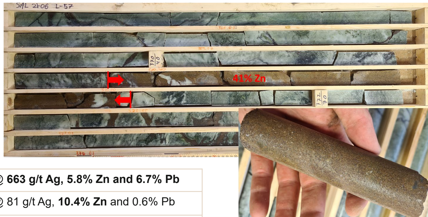
Figure 1: Half core from SAL2106 with 41% Zinc and 17 g/t Ag over 1.1m from 371.2m, part of larger interval of 14.0m @ 30 g/t Ag and 7.6% Zn from 365.5m 1 . Inset image illustrating close up of the massive sulphide sphalerite mineralisation.
